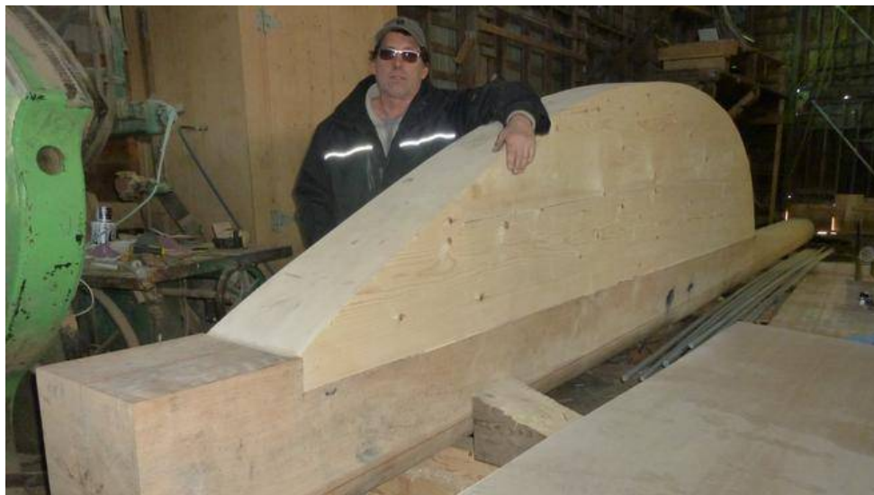
Snyder's Shipyard co-owner Wade Croft is dwarfed by the 25-foot rudder being constructed in Dayspring for the Bluenose II. (Peter Simpson)
